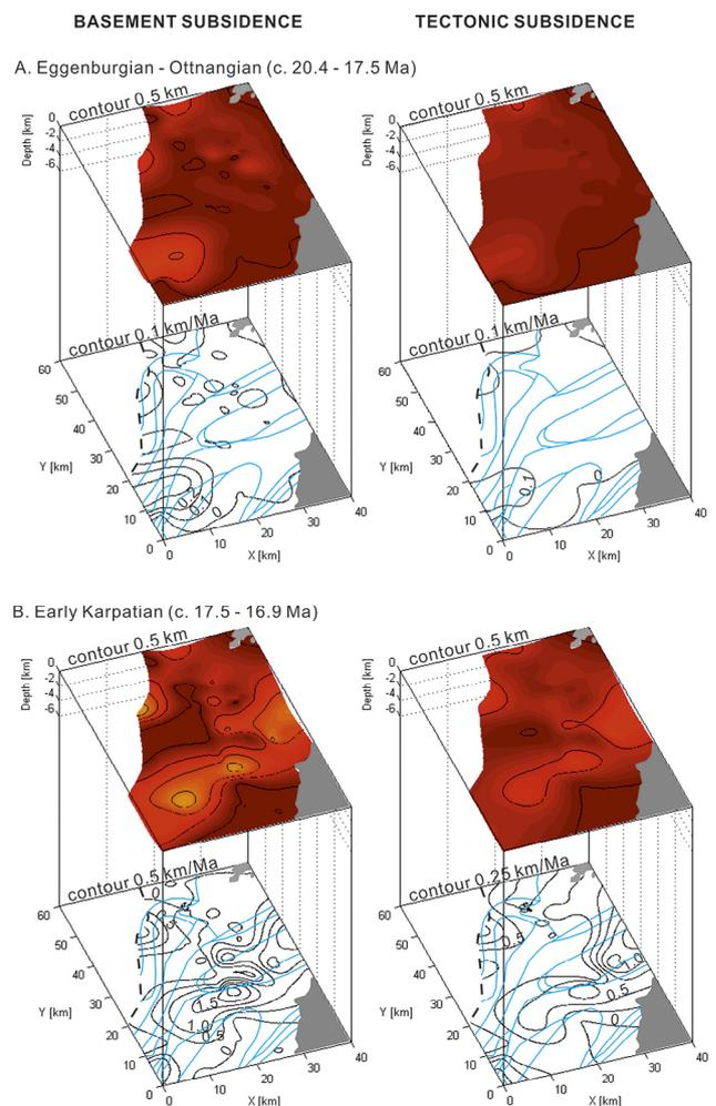
**Figure 9:** 3D subsidence depth (above) and subsidence rate (below) maps of the basement subsidence (left) and tectonic subsidence (right) visualized in the study area; A: Eggenburgian–Ottngian (c. 20.4 – 17.5 Ma) and B: early Karpatian (17.5 – 16.9 Ma). The Alpine-Carpathian thrust nappe borders are shown with blue solid lines and the location of the Steinberg fault with black broken lines.
