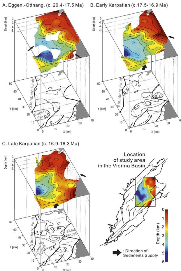
**Figure 6:** 3D sediment distribution surfaces (above) and sediment thickness isopach maps (below) of the Early Miocene visualized in the study area; A: Eggenburgian-Ottangian (c. 20.4 – 17.5 Ma), B: early Karpatian (c. 17.5 – 16.9 Ma), and C: late Karpatian (c. 16.9 – 16.3 Ma). The major faults and contour lines (0.5 km) are shown with black solid lines in the maps. Direction of sediment supply is from Sauer et al. (1992).
