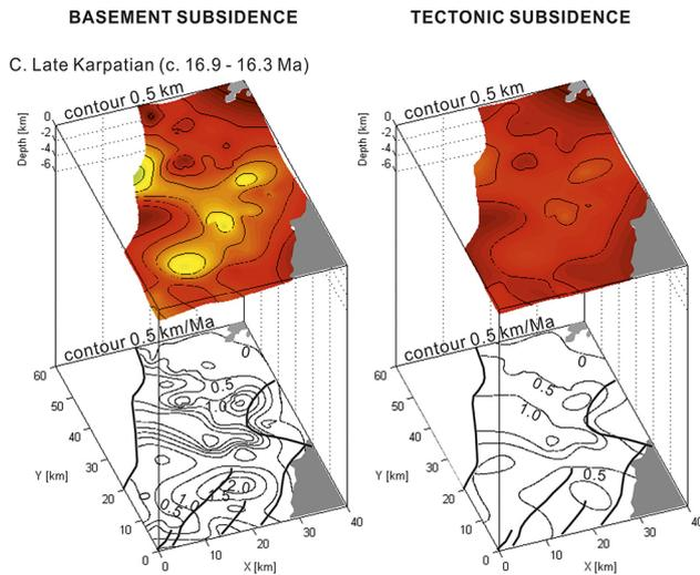
**Figure 10:** 3D subsidence depth (above) and subsidence rate (below) maps of the basement subsidence (left) and tectonic subsidence (right) visualized in the study area; C: late Karpatian (c. 16.9 – 16.3 Ma). The major faults are shown with black solid lines in the rate map.
