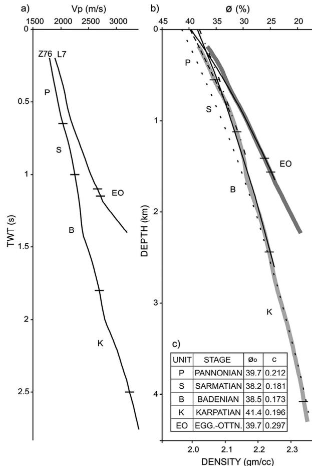
**Figure 5:** Porosity-depth relation evaluated for the Vienna Basin. a) Seismic velocity-Two Way Time (TWT) curves from locations of two wells (Zavod 76 and Lakšárska Nová Ves 7), b) Porosity and Density-Depth curves with exponential trend lines of each stage, and c) evaluated initial porosity ( $\Phi_0$ ) and coefficient (c) of each stage.
