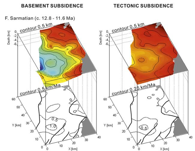
**Figure 12:** 3D subsidence depth (above) and subsidence rate (below) maps of the basement subsidence (left) and tectonic subsidence (right) visualized in the study area; F: Sarmatian (c. 12.8 – 11.6 Ma) and G: Pannonian (c. 11.6 – 7.8 Ma). The major faults are shown with black solid lines in the rate map.
