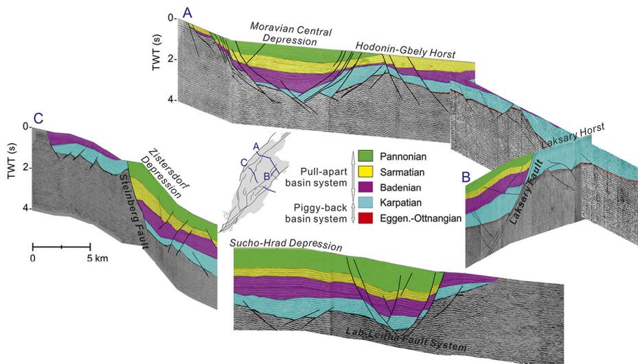
**Figure 3:** Seismic sections across the study area (see Figure 1 for location). Section A and C were revised from Čekan et al. (1990), and section B was acquired from the archives of the Dionyz Štur Institute, Slovakia. These sections were visualized by Blender which is an open-source 3D computer graphics software.
