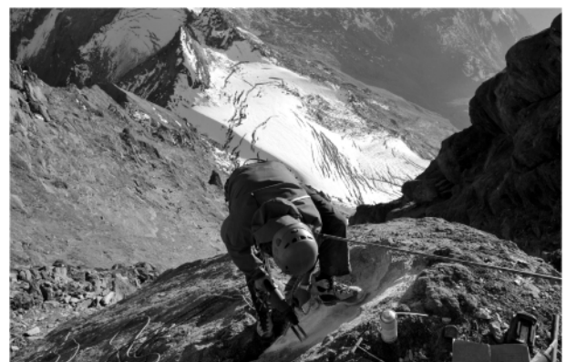
FIGURE 8: Drilling of a shallow borehole for iButton® temperature measurement at the Kitzsteinhorn south face (Photograph by Ingo Hartmeyer).
